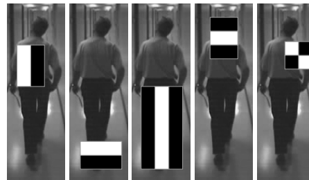
Figure 7. Examples of the five feature types we use. The position and size of the features with respect to the base window size of 48x16 are varied to define an overcomplete set of 8294 features.
