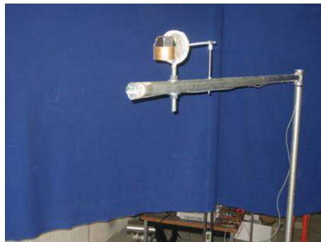
(a) Traffic pole with pounding TMD [20]
