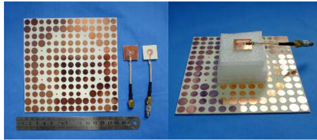
FIG. 6. Fabrication of the patch antenna and the gradient metasurface.
