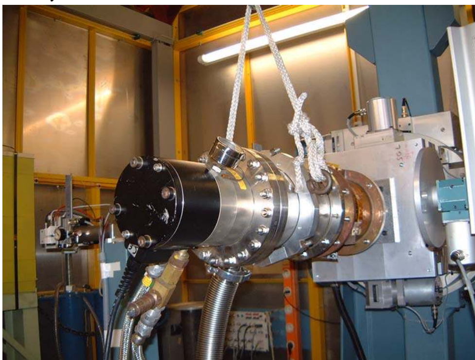
Figure 5-2 Close up of the Leybold RGD 1245 Cryostat at BW2, HASYLAB.
