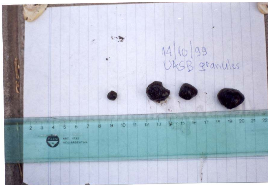
Figure 2. Granules observed in the UASB reactor fed with settled sewage.
