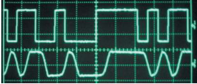
Figure 6-5: Oscilloscope traces of input to (top) and output from (bottom) a fifth order Chebyshev filter delay line
