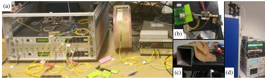
Figure 4. The experimental setup: (a) optical signal generation and fiber transmission, (b) PD and MPA connected to the transmitting antenna, (c) receiving antenna connected to the LNA, (d) the VSG and the DSO capturing the received signal traces.
