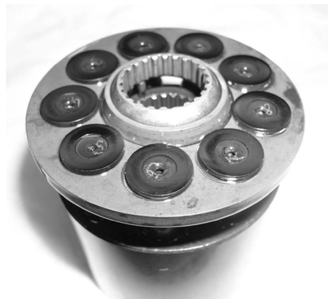
Fig. 3 Assembly of the pistons with DLC-coated shoes, inserted into the pump cylinder block
