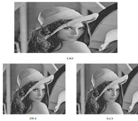
Figure 9. Vertical Pixel Interleaving. (a) Original Image (512x512) (b) SubImage 1 (512x256) (c) Sub-Image 2 (512x256)
