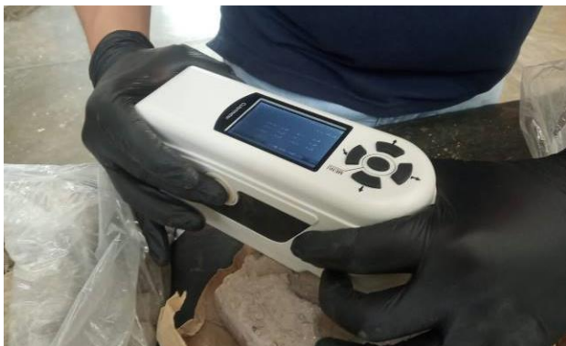
Figure 10. Use of the colorimetry equipment in an adobe sample. Photo: David Preciado Villicaña (2019). © SPOT Image Copyright 2020.
