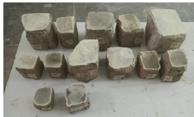
Figure 12. Adobe samples prepared for the compression test. Photo: Adrià Sánchez Calvillo (2019). © SPOT Image Copyright 2020.
