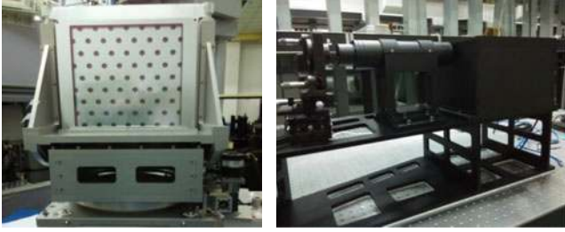
Figure 16. Deformable mirror (left) and Hartmann sensor (right) in AO system.
