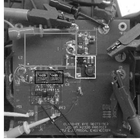
Fig. 14: Converter prototype with marked subcircuits. Gate driver (red), input filter (white), inverter (black), rectifier (green) and resonant tank 1 (cyan).
