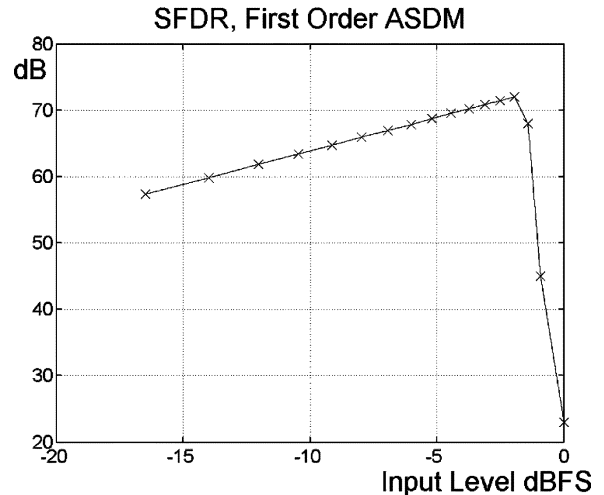
Fig. 14. SFDR with respect to the amplitude of the input signal.
