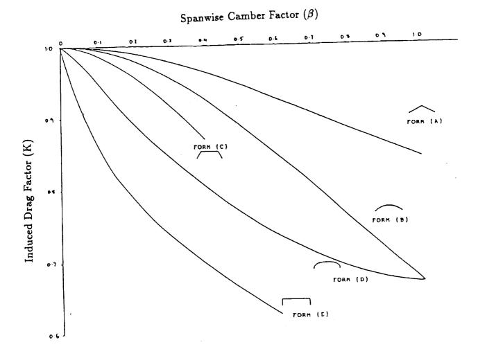
Figure 1: Variation of Minimum Induced Drag Factor with Camber Factor for 5 Forms of Vortex Arc. 13
