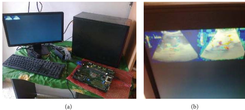
FIGURE 7: The FPGA output in the monitor through VGA. The first image shows the kidney portion segmented from the US image and second image witnesses the detected stone in that image indicated with red color.
