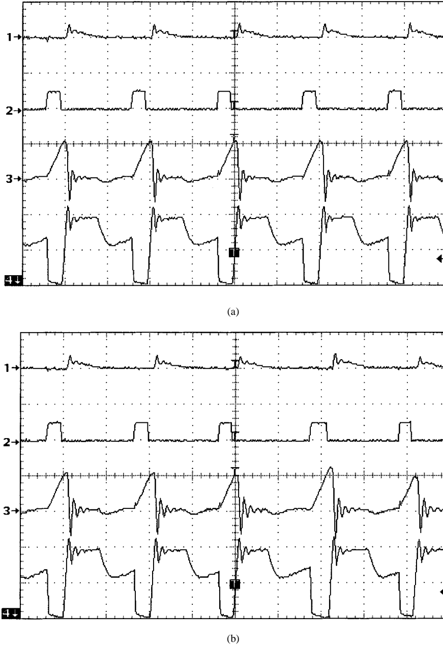
Fig. 4. Experimental waveforms of the converter. (a) \mathfrak{R} = 0 . (b) \mathfrak{R} = 0.2 . [Channel 1: Output voltage (1 V/div, with ac coupling). Channel 2: Gate signal (10 V/div). Channel 3: Input current (1 A/div). Channel 4: Switch voltage (200 V/div). Timebase: 10 \mu s/div.]
