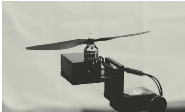
Figure 4. Testing device for the determination of propeller lifting force.
