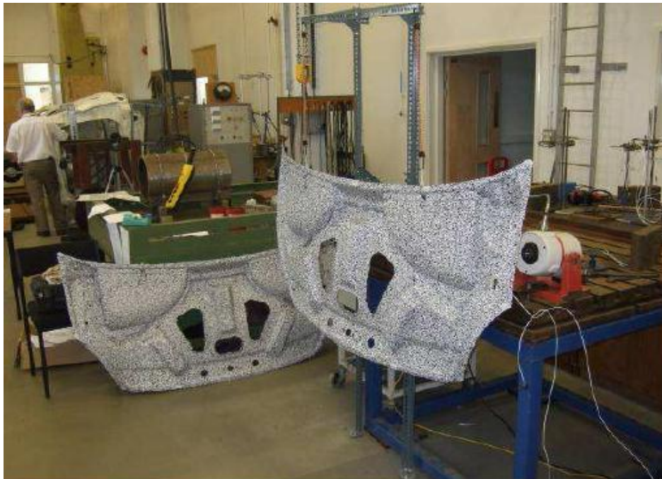
Figure 11: Bonnet structure with shaker [47]
