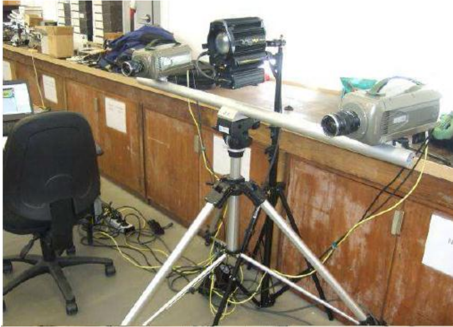
Figure 10: Setup of High speed DIC system [47]
