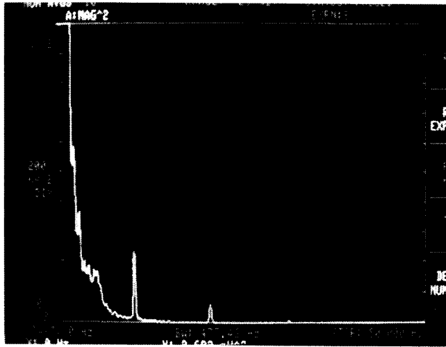
Fig. 17. Measured spectrum of the inductor current for a buck converter in continuous conduction mode with randomized PWM.
