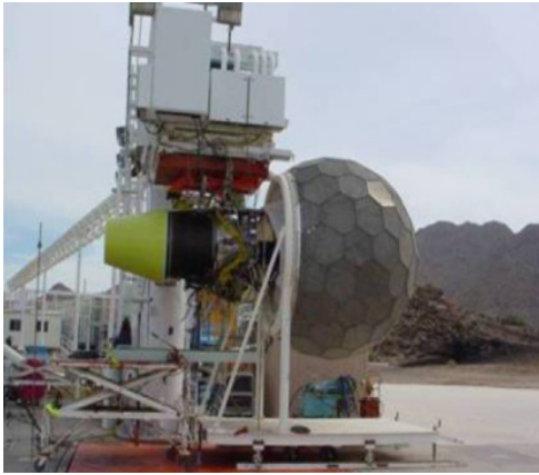
Figure 1. Photograph of the TECH977 engine mounted in the test stand. An inlet flow control device can be seen mounted around the engine inlet 3 .
