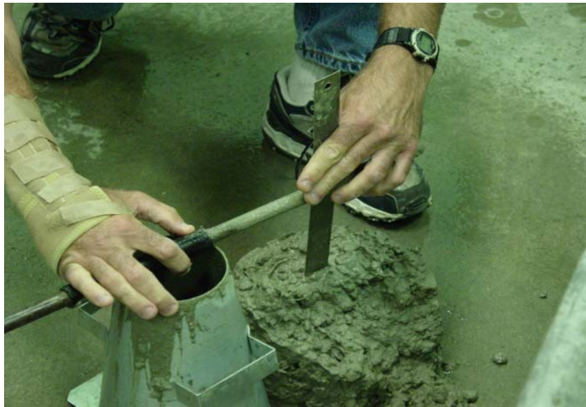
Figure 5: Slump testing concrete
