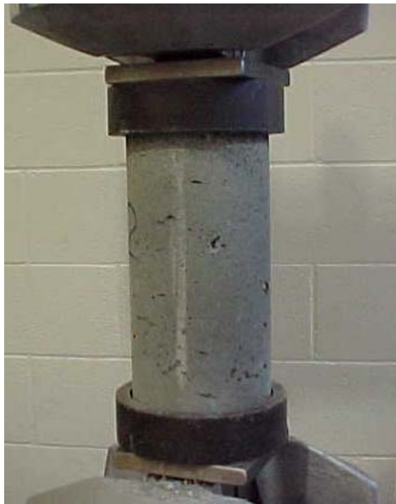
Figure 3: Concrete in compression test.
