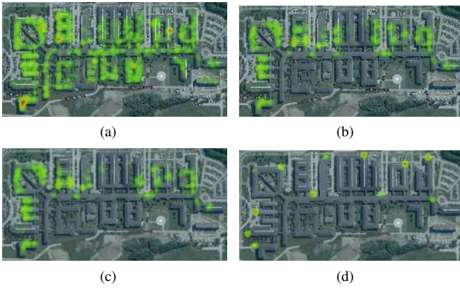
Fig. 8. (a) Heat-maps representing all device positions; (b) Only inside to outside movements (leaving the building); (c) Positions of filtered exits; (d) Estimated exits constrained to real exits.
