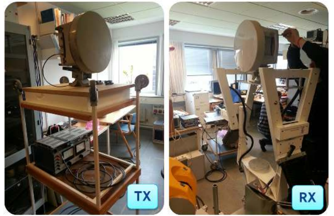
Fig. 2. Overview of antenna mountings at 1.75 m height on the manual-operated trolley (TX) and rotating pedestal (RX).
