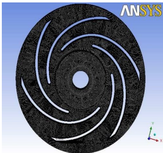
Fig.2 Unstructured mesh of the impeller
