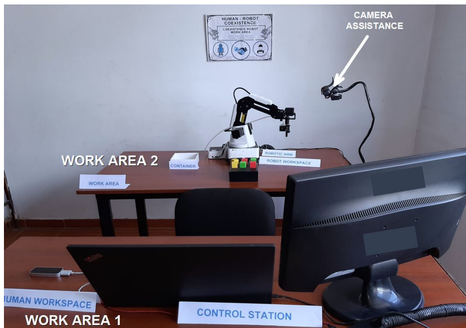
Figure 9. Human–robot workspace. Workspace 1 is the area where the user operates the robotic arm without line of sight to the robot. Workspace 2 is the area where object manipulation tasks are performed.
