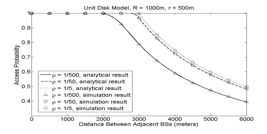
Access probability with L changing under the unit disk model, R = 1000m, r = 500m,  $\rho$  = 1/5, 1/50, 1/500 vehicles/m respectively.
