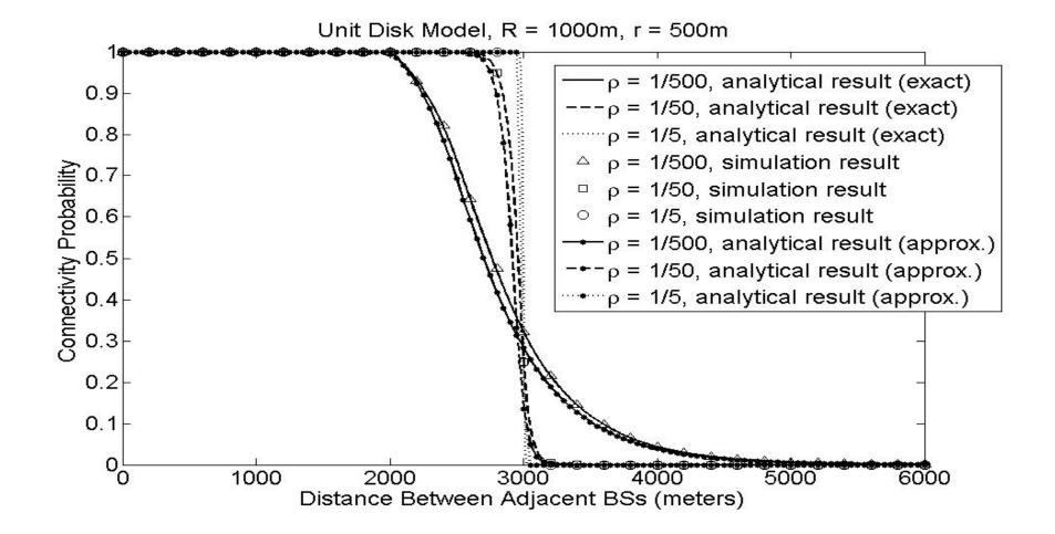
Connectivity probability with L changing under the unit disk model, R = 1000m, r = 500m,  $\rho$  = 1/5, 1/50, 1/500 vehicles/m respectively.
