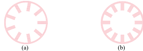
Fig. 14. Stator geometries. (a) 9-slot. (b) 12-slot.
