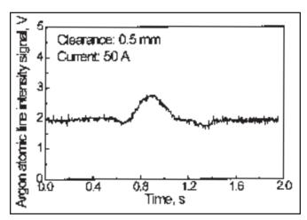
Fig. 17 — Line intensity signal in detecting a square groove in GTAW.
