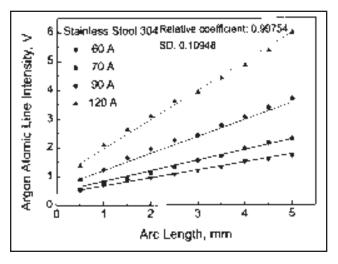
Fig. 10 — Argon atomic line intensity vs. arc length.
