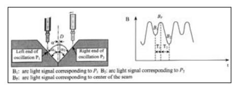
Fig. 14 — Monitoring of torch deviation based on arc light signal.
