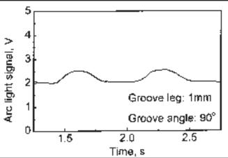
Fig. 15 — Arc light signal for detecting deviation of the welding torch.
