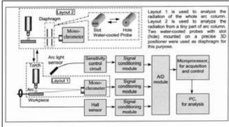
Fig. 2 — Experimental setup of the arc light radiation study.
