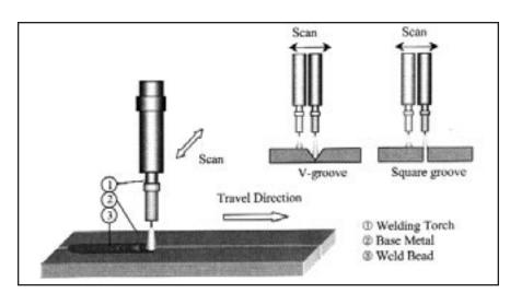
Fig. 13 — Arc light signal for detecting deviation of the welding torch.
