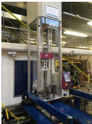
Figure 3. INSTRON CEAST 9350 drop tower used to damage the panels
