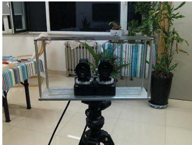
Figure 7. The physical diagram of the auto-converged camera array.
