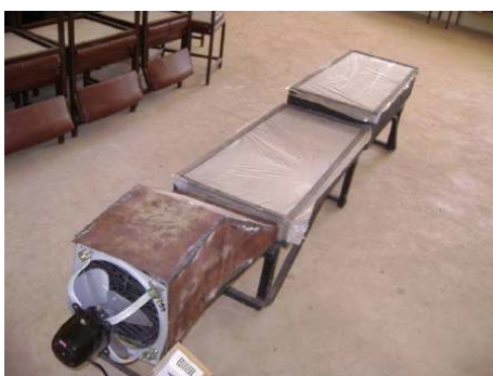
FIGURE 10: Showing the diagram of a solar dryer. Source: Propcom [21].
