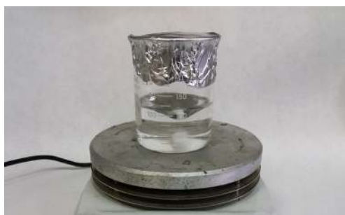
Figure 4. Paraformaldehyde dissolution using magnetic stirrer with hot plate
