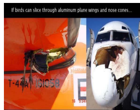
Bird strike through nose cones of aero plane
