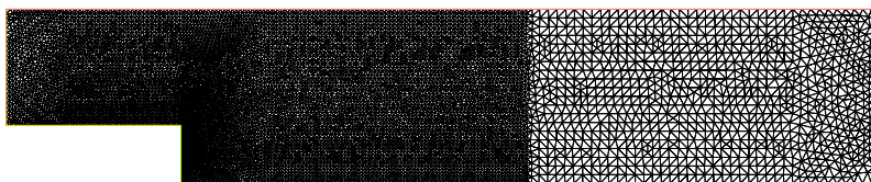
FIGURE 2. Triangular mesh of the channel - 16 425 triangles and 8 846 vertices.
