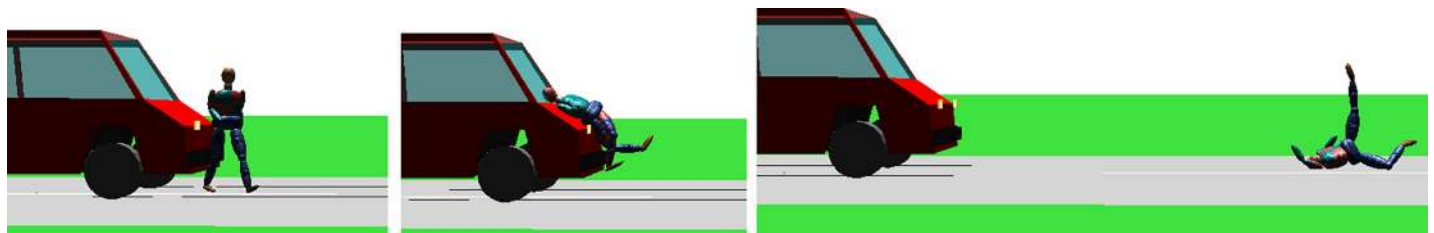
Fig 4. Posture of the pedestrian after collision. (A) t = 0.020 s. (B) t = 0.100 s. (C) t = 1.119 s.
