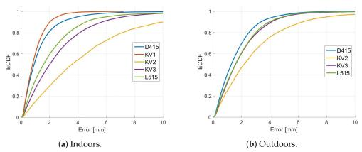
**Figure 14.** Plots comparing ECDF plots for scans of two different unpainted grape bunches which were captured by depth cameras (**a**) indoors and (**b**) outdoors in direct sunlight using ICP alignment of the depth camera scans with the photogrammetry scans. The grapes were located 600 mm from the cameras.
