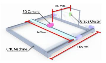
**Figure 1.** Diagram showing setup of camera and grapes mounted onto the CNC machine for capturing RGB-D images.
