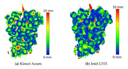
**Figure 9.** Kinect Azure and Intel L515 error scans for unpainted grapes after the depth camera scans were aligned with the photogrammetry reference scan using the ICP alignment method.
