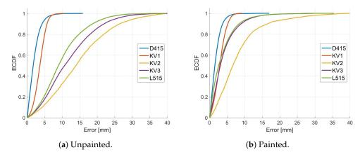
**Figure 12.** Plots (**a**,**b**) respectively show the ECDF error measurements for the grape bunch scans made indoors before and after the grapes had been sprayed with paint. The cameras were positioned 600 mm from the grapes.
