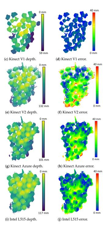
**Figure 7.** Depth and error scans (relative to the photogrammetry scans) for the RGB-D cameras located indoors at a distance of 600 mm from the unpainted grape bunch. An error bar is provided that shows the colour scale for the error scans and is the same for all the cameras. The colours for the depth scans are relative to the maximum and minimum depth of the point cloud for each camera.
