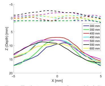
**Figure 11.** Plots showing cross-sections of scans made by the Kinect Azure of a single grape before (solid lines) and after (dashed lines) the grape had been painted. The different colours represent scans made with the camera being located at distances from the grape ranging from 350 to 600 mm.
