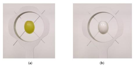
**Figure 4.** Photos of the setup of scans for a single grape which is first unpainted (**a**) and then painted (**b**). This was performed to analyse the effect of diffused scattering within the grape for the RGB-D cameras, which use ToF and LiDAR technologies.
