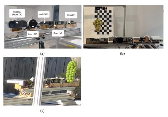
**Figure 2.** Photos of the experimental setup. Photo (**a**) shows the front view of the cameras mounted onto the 2D gantry. Photos (**b**,**c**) respectively show the setup located inside and outdoors.
