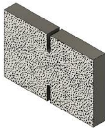
(a) Illustration of a specimen surface. (b) Type II specimen with applied speckle.
