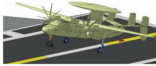
FIGURE 7: Carrier-based aircraft landing virtual prototype.
