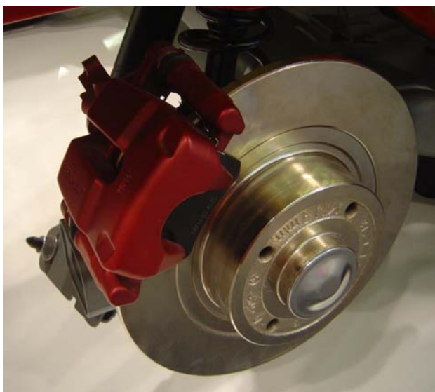
Fig. 1 Disk brake rotor, pad, and caliper assembly
