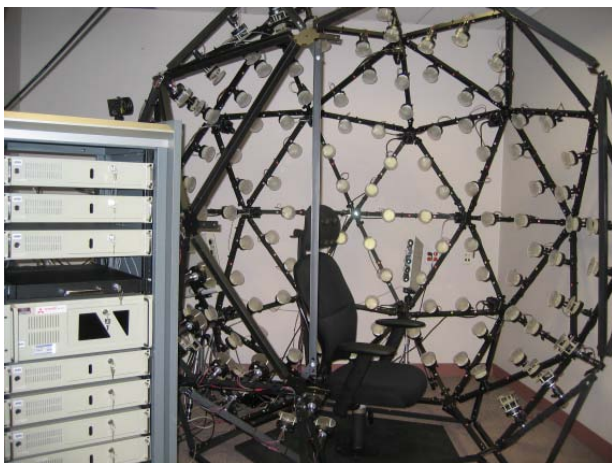
Figure 4: The face-scanning dome consists of 16 digital cameras, 150 LED light sources, and a commercial 3D face-scanning system.
