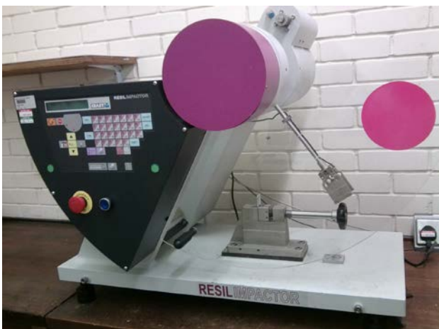
Fig. 1. Resil impact test set-up with GFRP specimen
