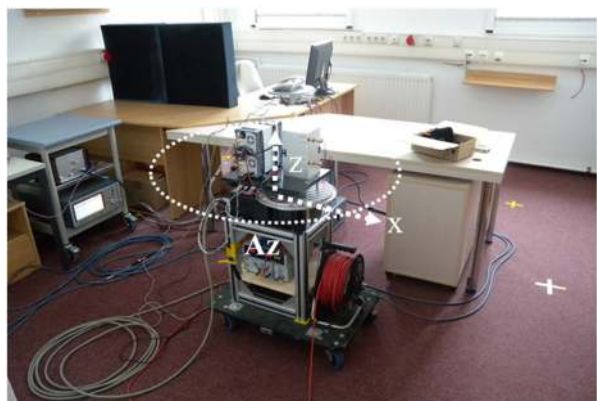
Fig. 3 RX mounted on the rotational positioner at position 2 in the office. Angular coordinates are overlaid in white
