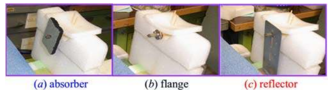
FIGURE 9. Open-ended waveguide probe antenna with a flange covered by an absorber and a reflector.
