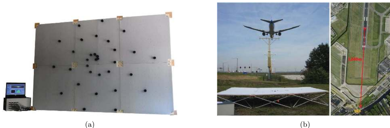
Figure 1: (a) 32 Microphone array configuration, (b) Experimental setup located 1240 m to the South of the threshold of the Aalsmeerbaan (36R) Schiphol airport runway.
