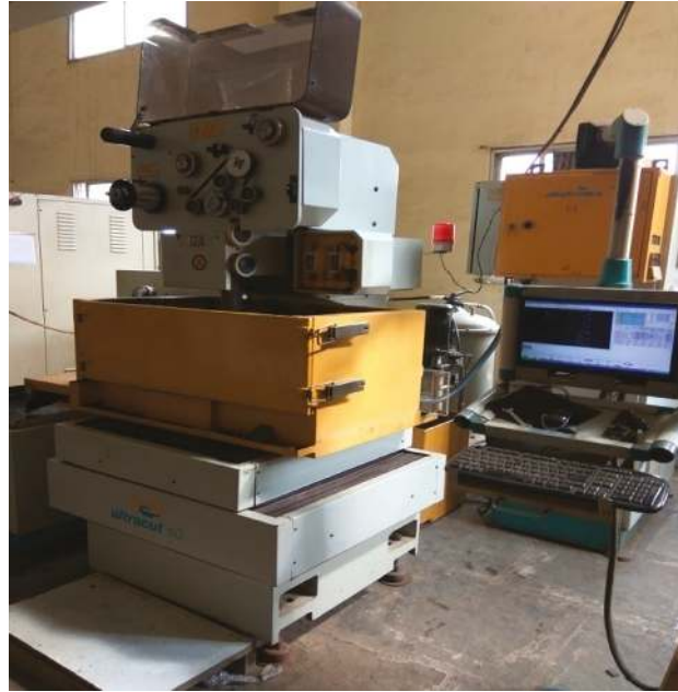
FIGURE 3: WEDM tool used for experimentation.
