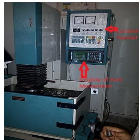
Figure 3.1 : Set-up of Electrical Discharge Machine
