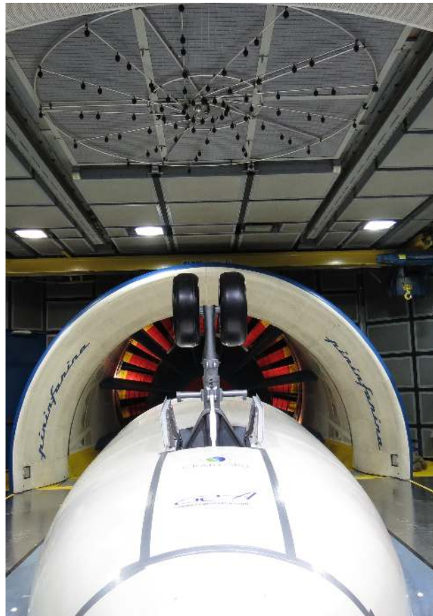
Figure 2: ALLEGRA NLG model inside the wind tunnel with the top array visible [41].
