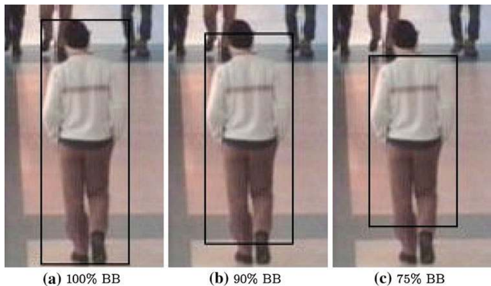
Fig. 3 Example of the height variation of the bounding box. In the left image , full bounding box is used; the bounding box is scaled down from left to right (sample frame of the CAVIAR project [11])
