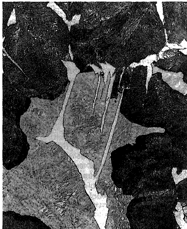
Figure 6 Microstructure of a Fe-0.57 mass % C alloy quenched from 940 K after cooling at a rate of 20 \text{ K min}^{-1} from a temperature of 1270 K, showing ferrite, pearlite and martensite.
