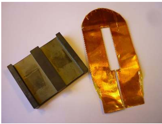
Fig. 10. Pictures of E64 core and realized winding (a) and assembled transformer (b).
